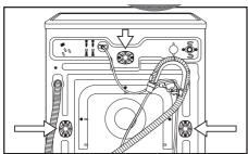
Loosen and remove the 3 blocking screws.
